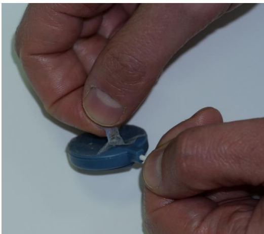
Figure 24 – Chest sensor sticker removal
