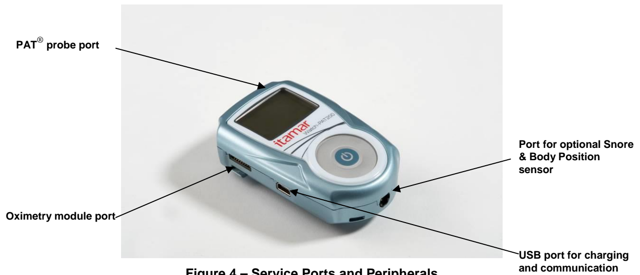
Figure 4 – Service Ports and Peripherals
