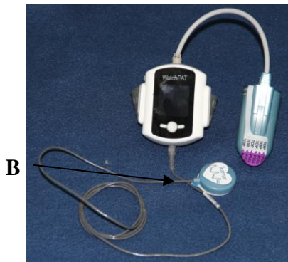
B - Integrated RESBP sensor
