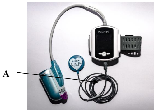
A - Integrated RESBP sensor
