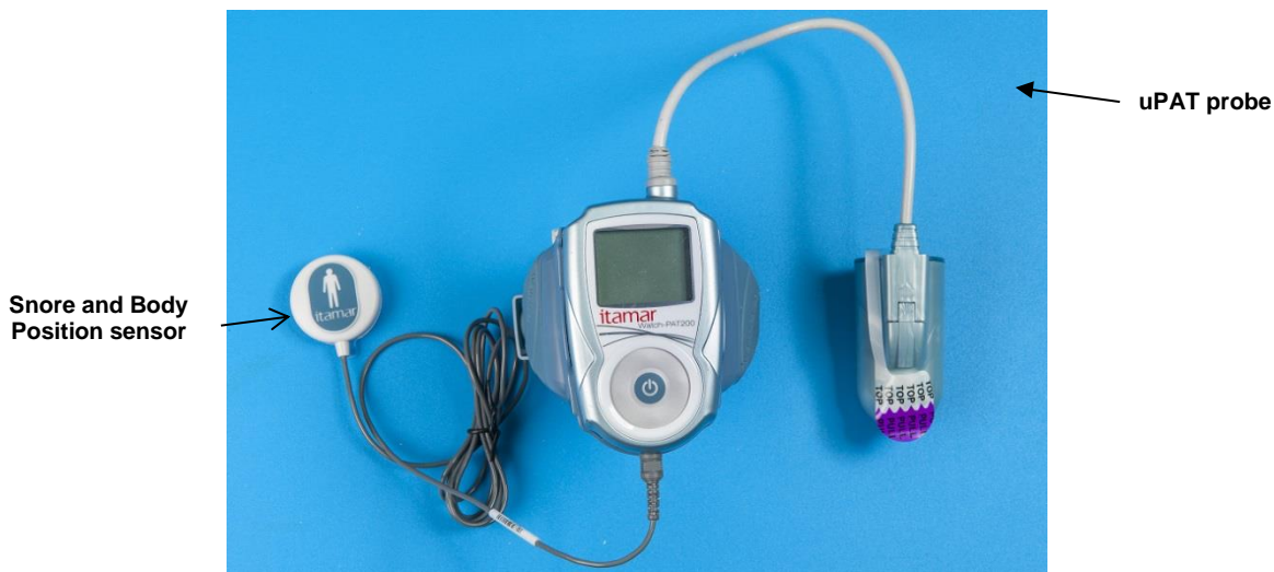
Figure 9 – WatchPAT™ Fully Prepared
