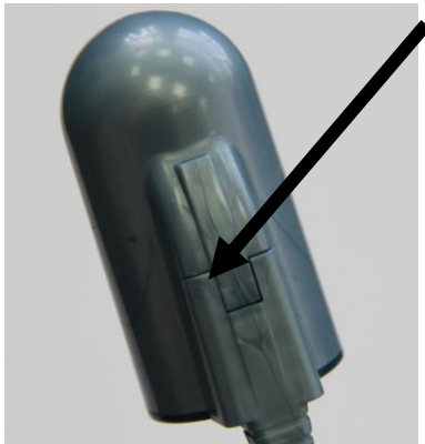
Figure 7 – Disconnecting the Probe
