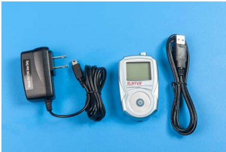
Figure 6 – Charging the WatchPAT™ Device
