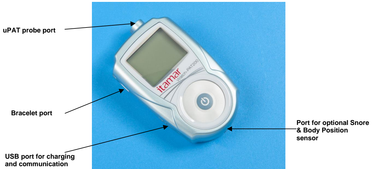
Figure 4 – Service Ports and Peripherals
