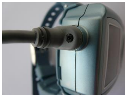
Figure 17 – uPAT Probe Cable with Screw
