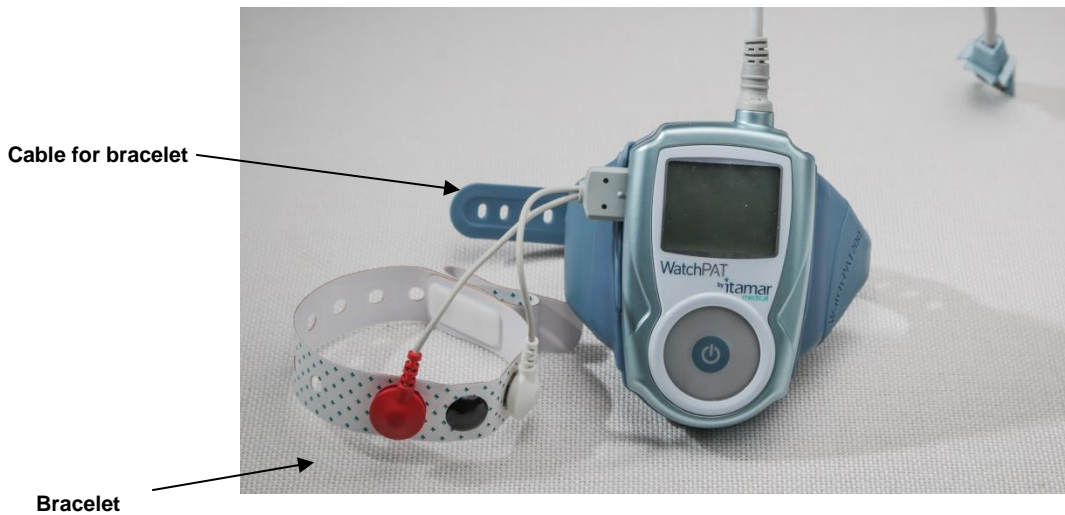
Figure 10 – WatchPAT™ Device with Tamper-Proof Bracelet
