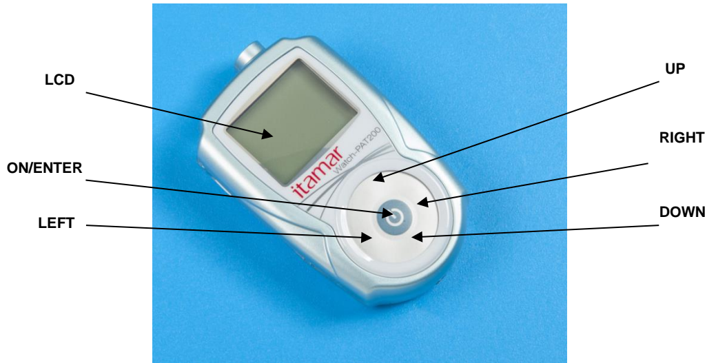
Figure 3 – The Buttons and Display
