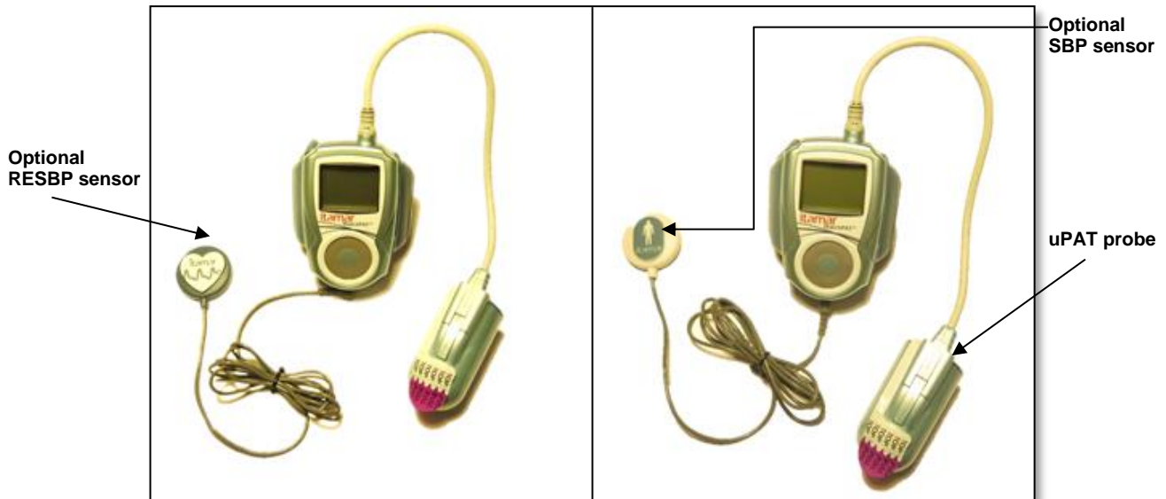
Figure 2 – WatchPAT™200U Device with Sensors
