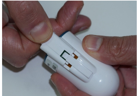
Figure 23 – New Finger probe connection
