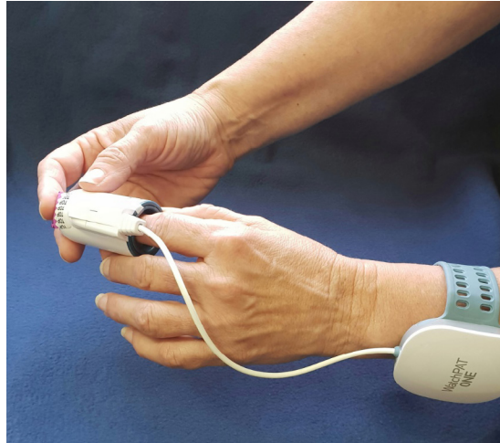
Figure 7 - Placing Finger in the Finger Probe
