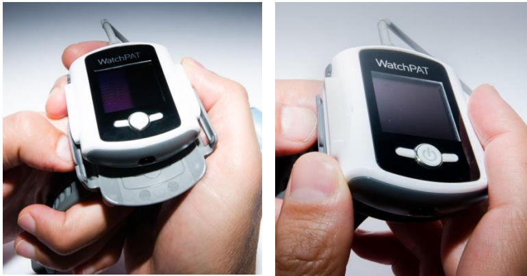
Figure 20 – Seating device on wrist strap
