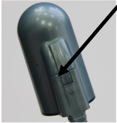
Figure 6 – Disconnecting the Probe
