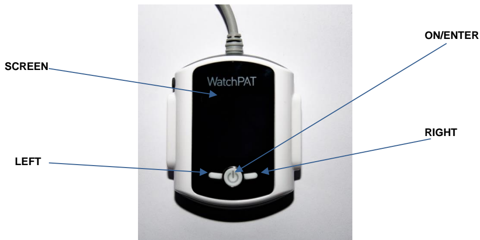
Figure 3 – The Buttons and Display
