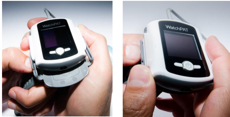
Figure 20 – Seating device on wrist strap
