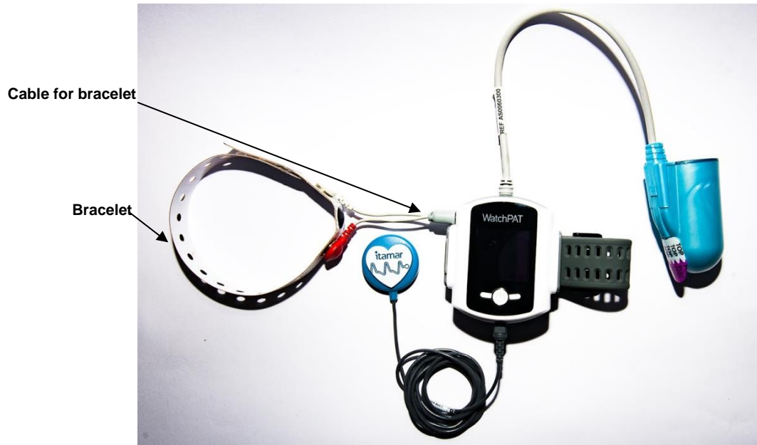
Figure 9 – WatchPAT™ Device with Tamper-Proof Bracelet
