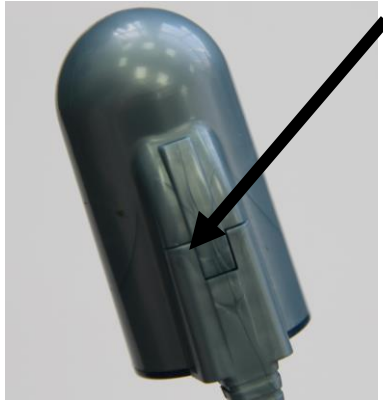
Figure 6 – Disconnecting the Probe
