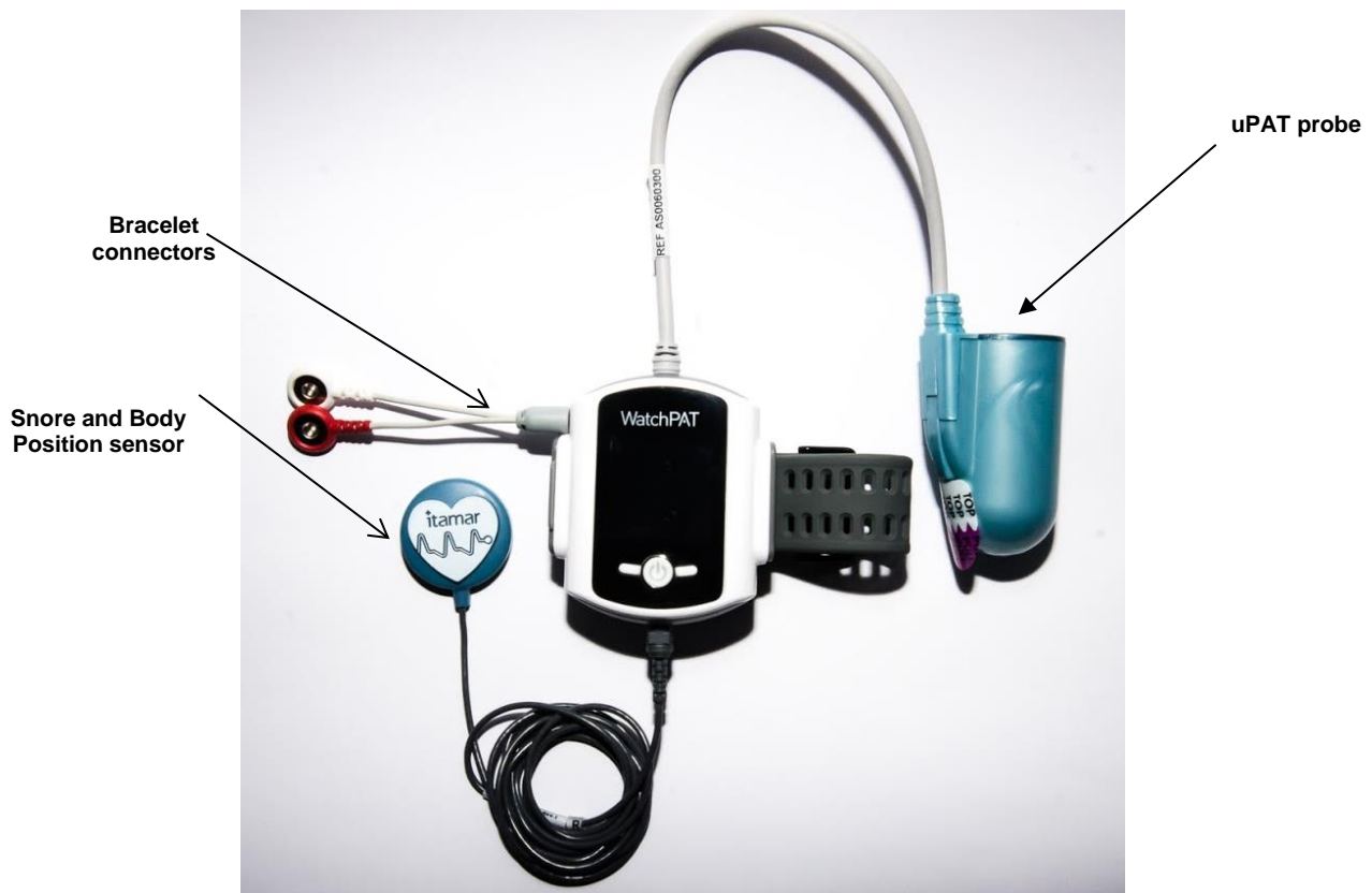
Figure 8 – WatchPAT™ Fully Prepared
