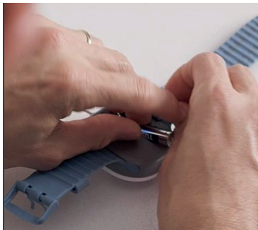
Figure 27 – Insertion de la pile
