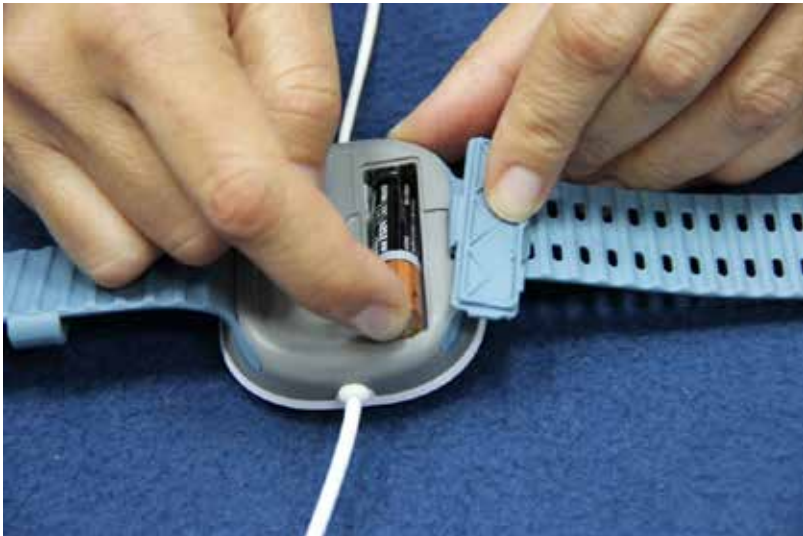
Figure 4 – Insertion de la pile
