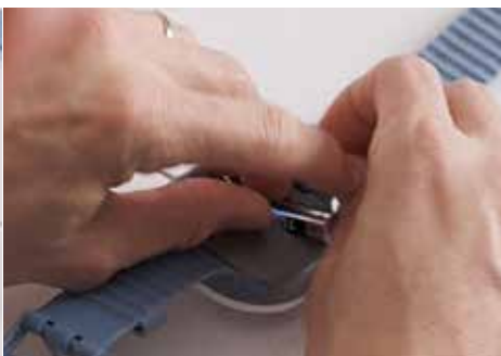
Figure 29 – Insertion de la pile
