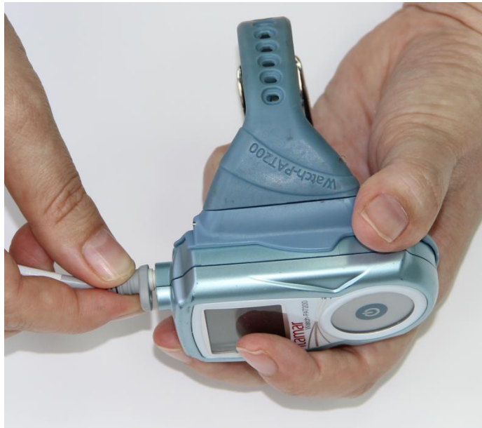
Figure 18 – Replacing the uPAT Probe
