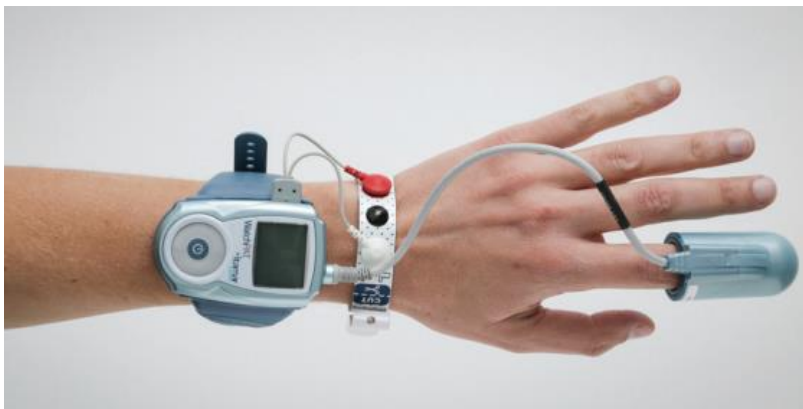
Figure 14 – Bracelet and WatchPAT™ Device on a Patient's Hand
