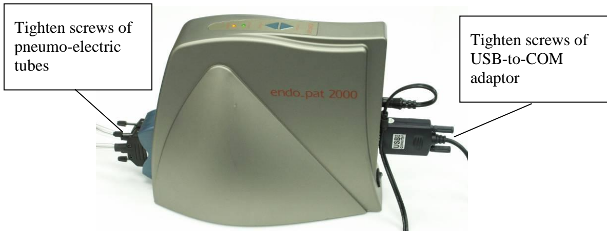
Figure 3 - Connection of pneumo-electric tubing and USB adaptor
