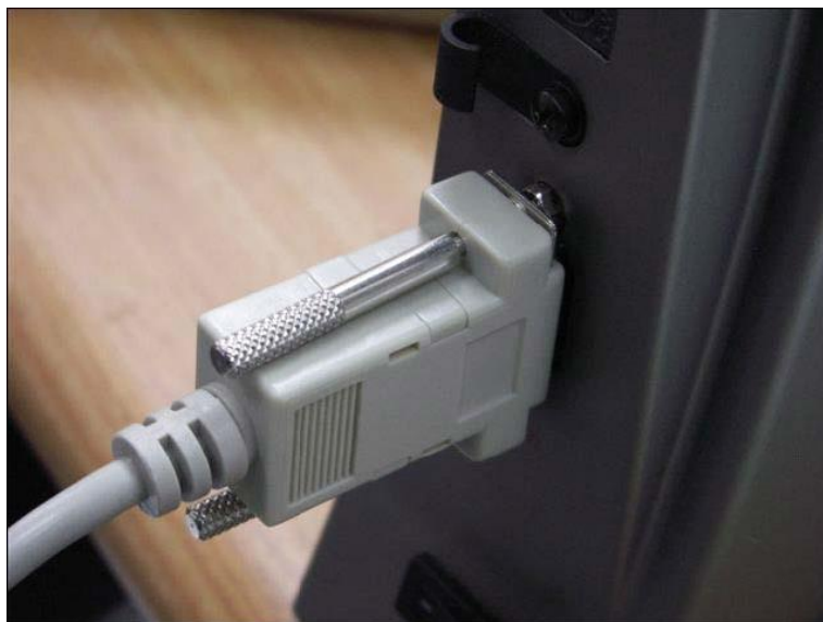
Figure 71 – connect COM TO COM
